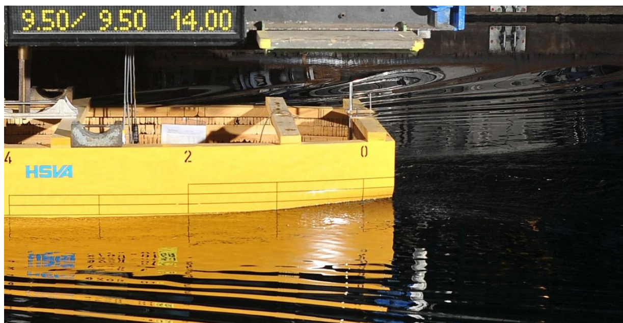
Wave formation at stern and behind the ship at 14 knots.
